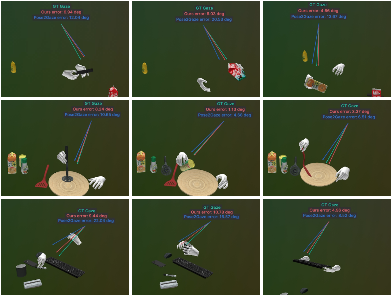
Fig. 4. Visualisation of the gaze estimation results from our method and the state-of-the-art method Pose2Gaze [Hu et al. 2024a] on the HOT3D dataset. The green arrow represents the ground truth eye gaze, the red arrow denotes our method, the blue arrow refers to Pose2Gaze . Our method exhibits higher estimation accuracy than the state-of-the-art method at different scenarios and different activities.
